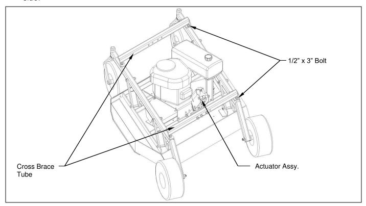
Figure 3. Cross Brace Tube Installation
