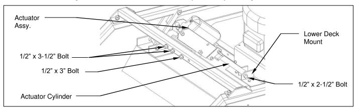
Figure 2. Actuator Assembly Installation
