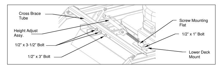
Figure 1: Manual Crank Height Adjust Assembly Removal
